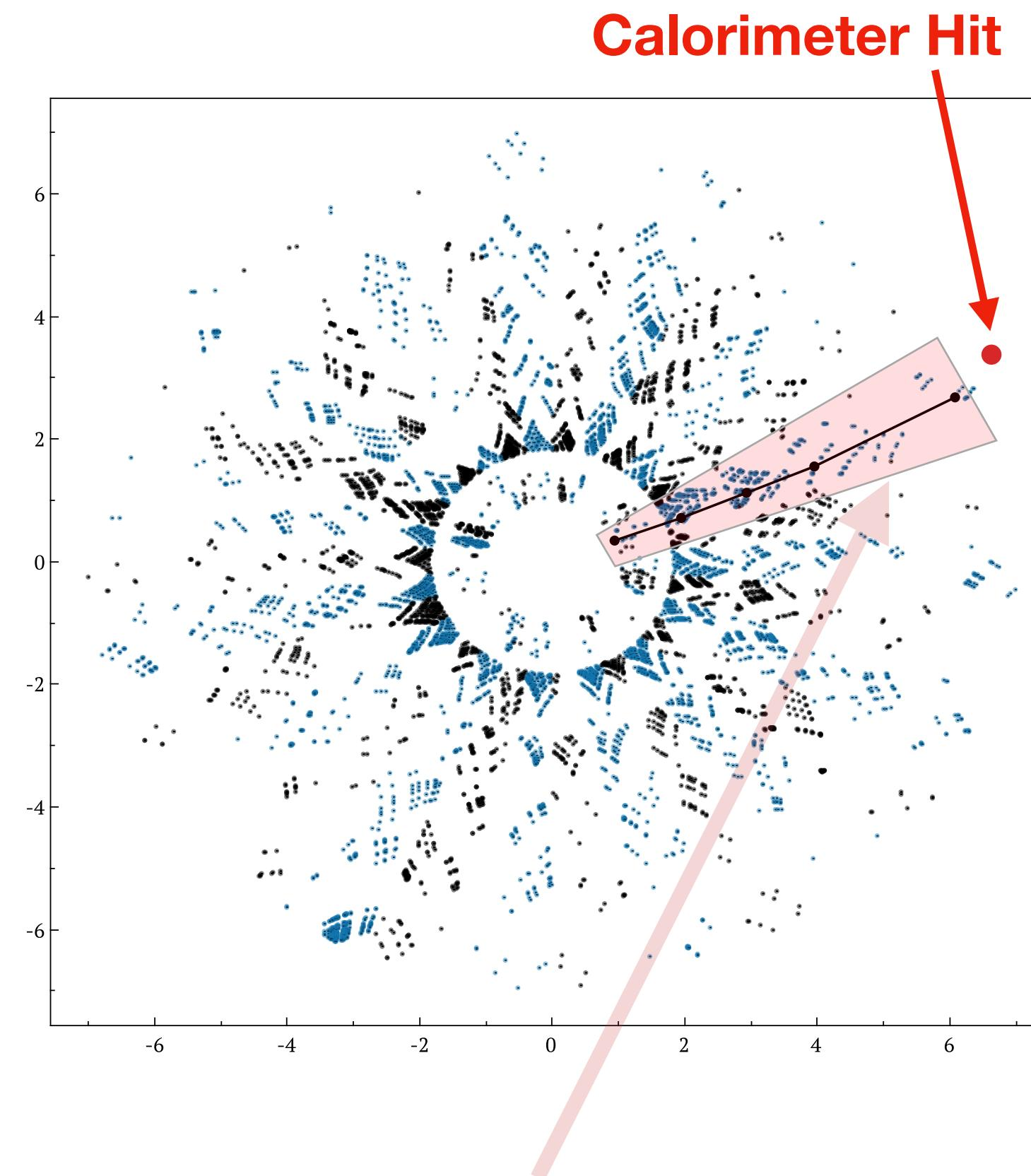
The Narrow region matching the position of the calorimeter hit is considered for training and track identification.
