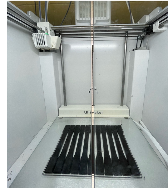
Fig: 3D Printer with dogbones
