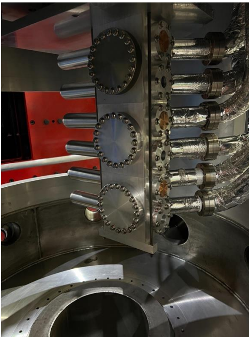
Target ladder with cryotarget cells.
