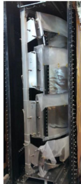
Cylindrical Mirrors Inside GRINCH
