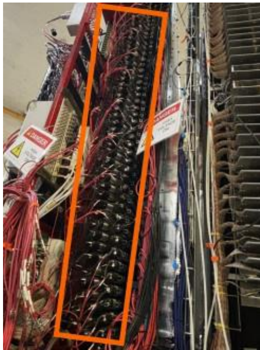
Zoom-in of Timing Hodoscope in BigBite Spectrometer
