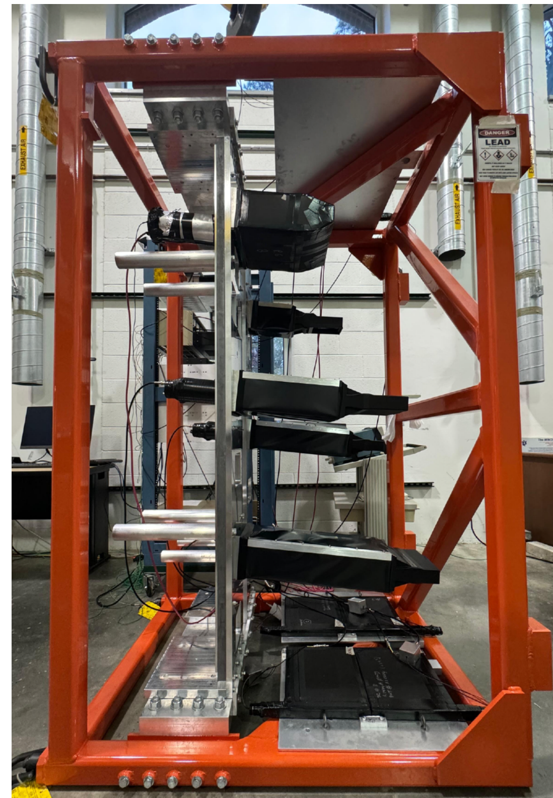
thin quartz assembly modules in cosmic test stand
