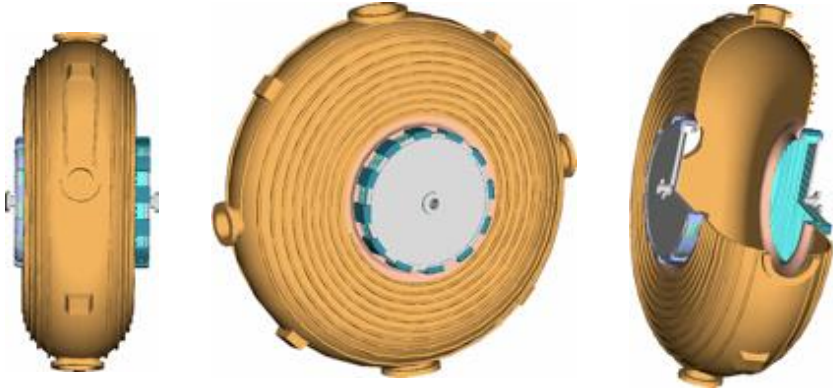
201.25 MHz cavity conceptual design
