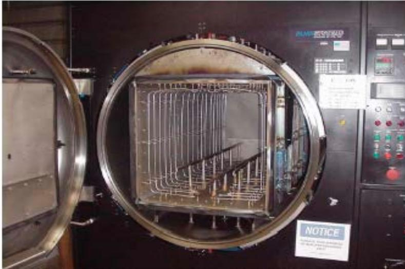
The standard furnace used for the high-temperature heat treatment of SRF cavities is an ultra-high-vacuum furnace with molybdenum hot-zone; molybdenum (or tungsten) resistive heating elements and cavities are heated by radiation from the heating elements.
