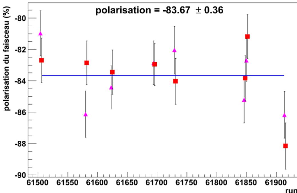
Beam polarization measurements during CLAS-EG6 run period. The red squares are the measurements with negative current in the Helmholtz coils of the polarimeter, while the purple triangles were with positive current. The figure is taken from the Y. Perrin, "Etude de la structure partonique du noyau d'hélium", CLAS-thesis, 2012.
