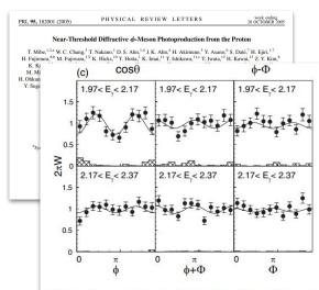
FIG. 4. Decay angular distributions for  $-0.2 < t + |t|_{min}$  in the Gottfried-Jackson frame. The solid curves are the fit to the data. The hatched histograms are systematic errors.
