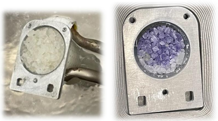
Ammonia crystals unexposed to beam (left), crystals after beam exposure (right). Purple color from paramagnetic centers.
