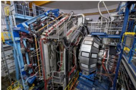
Fig. 1 The CLAS12 experiment in Hall B at Jefferson Lab. The photograph shows the CLAS12 detector complex. The overall extension of CLAS12 in the horizontal direction is about 13 m. Click on this link to view a video on the experiment.
