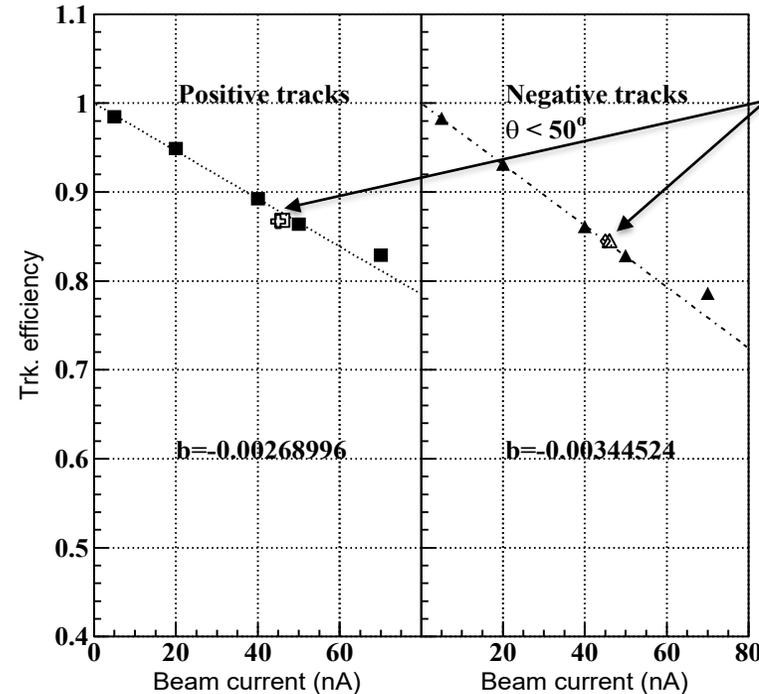
5 nA data merged with a beam background from 40 nA random trigger data.
