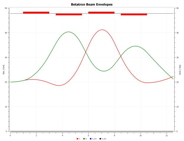
Red bars are 200 cm long, 416 mm ID quadrupoles. Muon beam radius assumed 20 cm. First quad is 100 cm from the concrete. Quad spacing 12 cm coil to coil. Beam divergence exiting from concrete NOT included Red horizontal, green vertical Peak radius 40 cm so there will be lots of clipping. One could also use a triplet, reducing length from 12 m shown.
