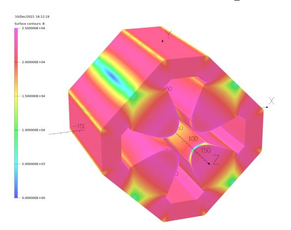
Opera's "good magnet steel" BH curve used. 300 A/cm² in coil. Pink is 2.5T on surface. If yoke thickness is increased from 30.5 to 40 cm, peak in yoke decreases to 2T and integrated focusing increases 3%. Field in pole doesn't change significantly. Not cost effective.
