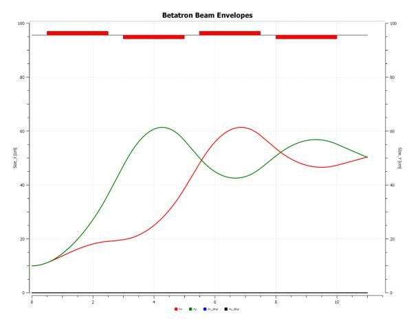
Limited by focusing strength available with steel. Peak radius 60 cm so clipping much greater yet than 2 GeV.
