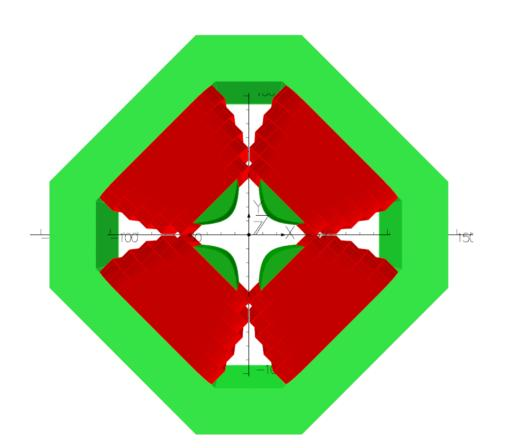
Luvata 8549, 11.5 mm square with 8.5 mm round hole, chosen as conductor. Using an online pressure drop calculator without bends, 150 g/s of water is driven by 12.7 bar in longest double pancake. Temperature rise at 300 A/cm² then ~42 C. Resulting field integral at 1 cm radius 130000 G.
