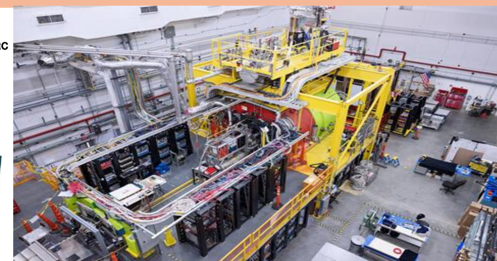
Figure 2: (Left) A diagram of the experimental setup in Hall D [2]. (Above) Image of the detector in Hall D as taken in 2024 [3]. Tracks measured by the detectors are used in decay reconstruction.
