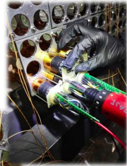
Using a torque screw driver: setting = 2
