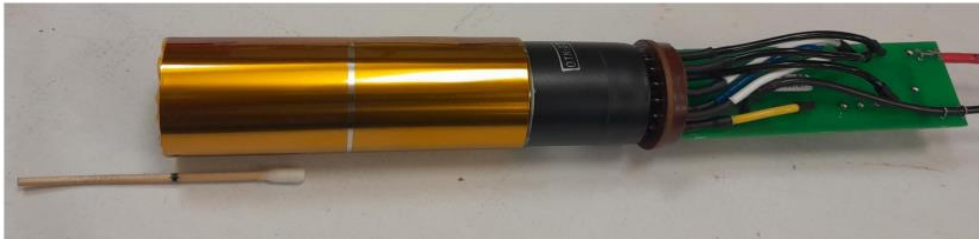
Assembled base, PMT and mu-metal
