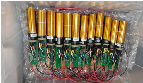
Assembled base, PMT and mu-metal
