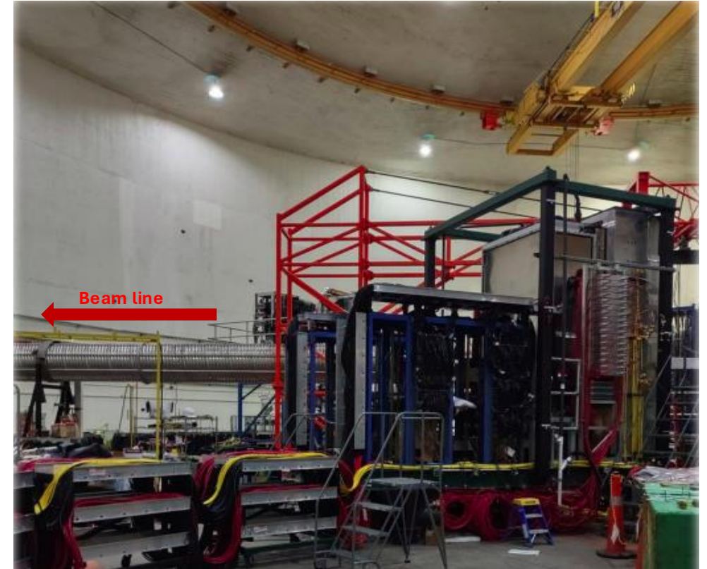
Figure: ECal (1656 channels) for SBS GEp V Experiment
