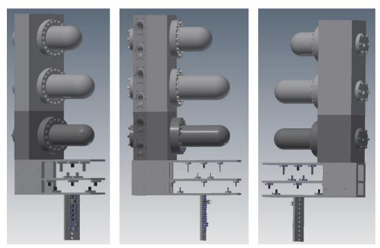
CAD views of the cryogenic and solid target ladders Jefferson Lab Hall C Standard Equipment Manual
