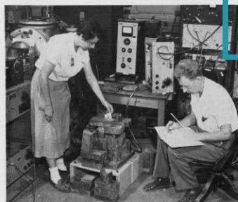
DETECTING RADIOACTIVE DECAY OF THE NEUTRON —The detection is achieved by means of the complicated apparatus shown above. Miss Frances Pleasonton, left, and Dr. A. H. Snell are shown checking the performance of the coincidence circuits. In this photograph, the neutron decay apparatus has been moved away from the pile face to a room with lower radiation background. The coincidence counters have been temporarily built into the pile of lead bricks in the center. Miss Pleasonton is inserting a radioactive source which is used for testing purposes.
