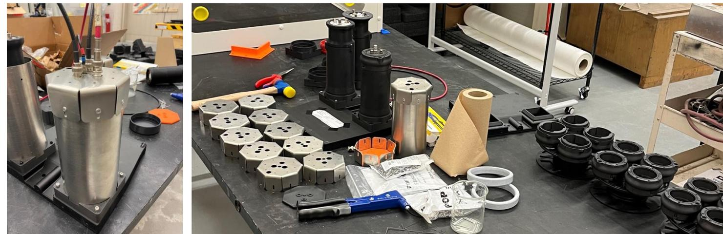
Fig: (left) LAM prototype, (right) 3D printed and aluminum components for LAMs
