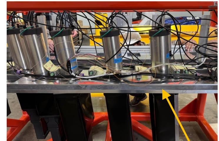
Fig: Segment frame: aluminum lead sandwich
