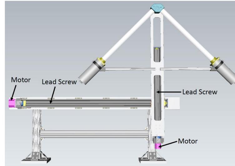
Fig: CAD assembly of upstream scanner
