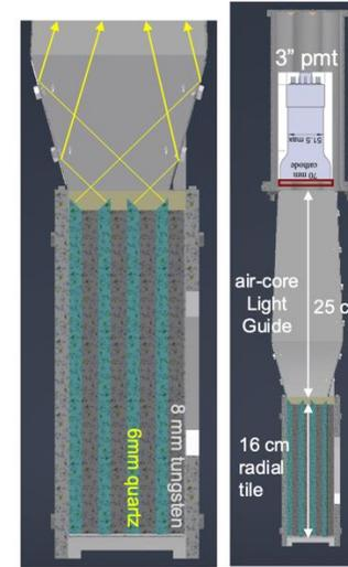
Fig: Cross section view
