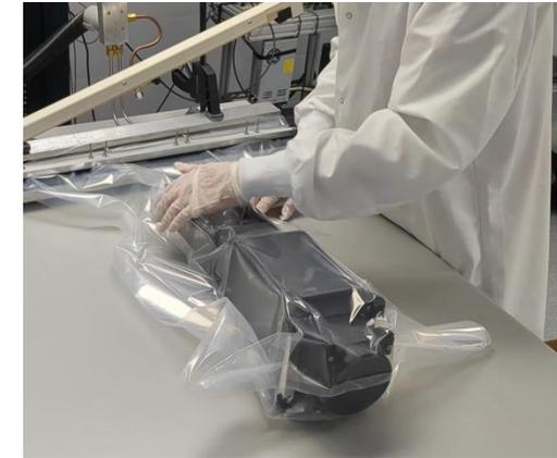
Fig: Vacuum sealing the module
