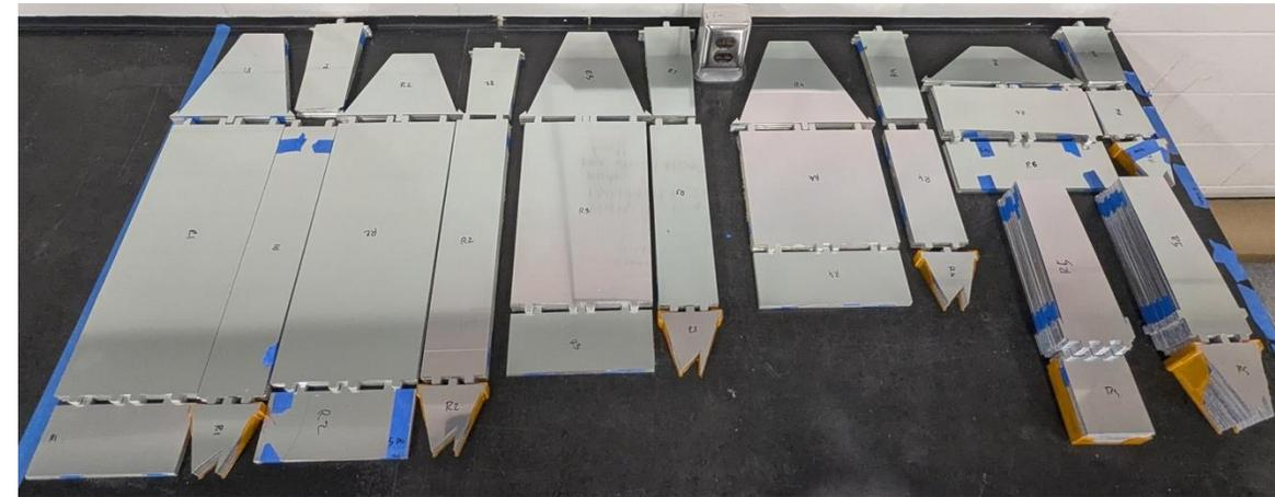
Fig: Laser cut aluminum light guides for all rings (R1 – R6).
