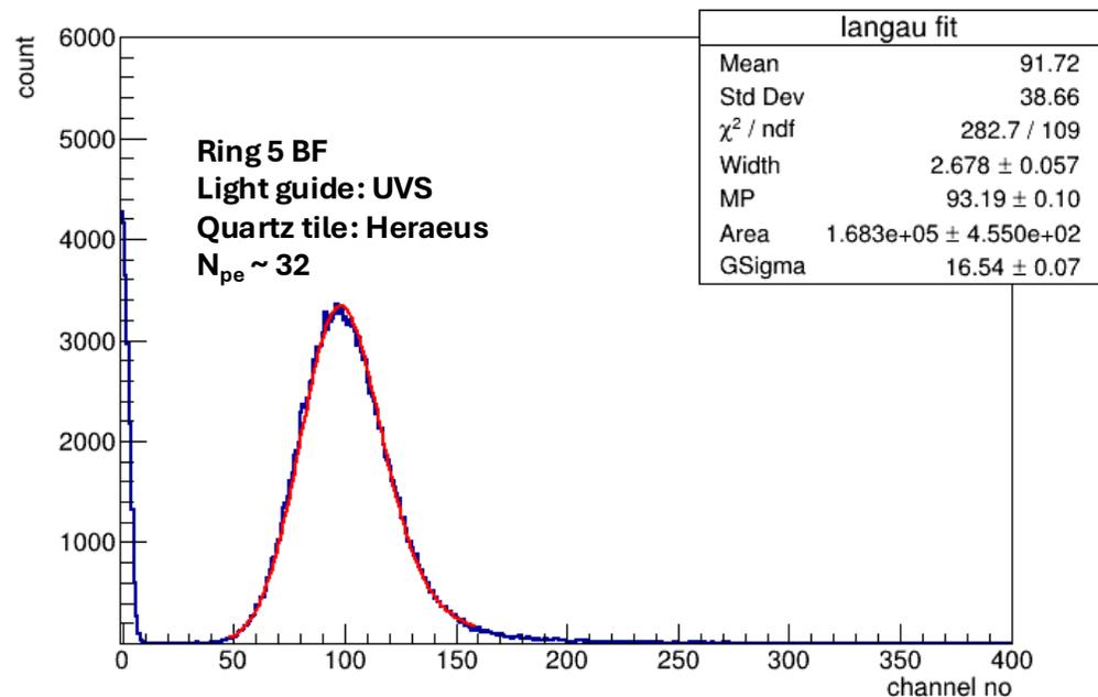
Fig: Pulse height distribution of the R5 detector
