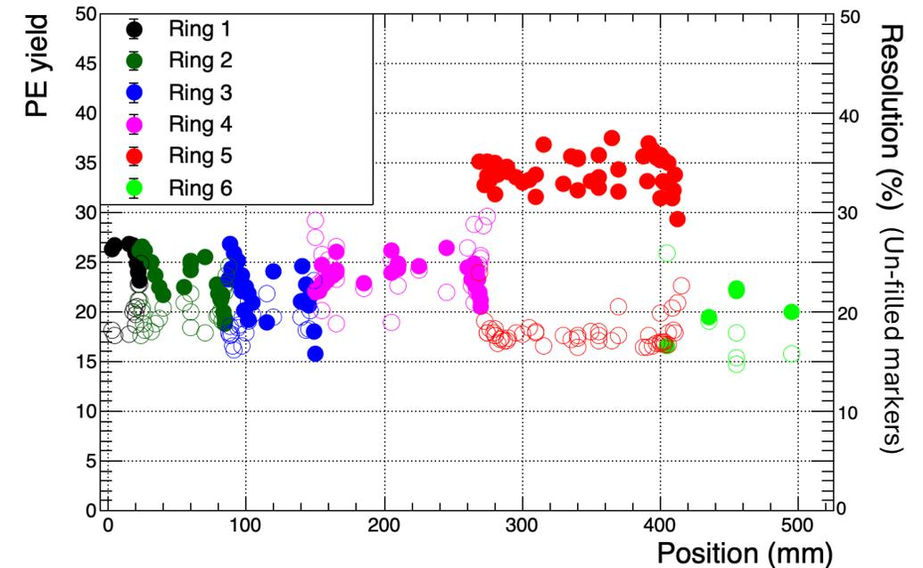
Fig: PE and Resolution vs radial position for R1-R6 detectors
