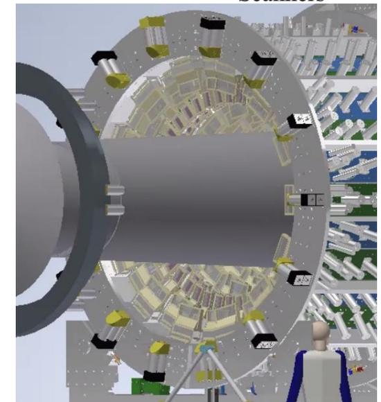
Fig: 14 DBMs around the beam line
