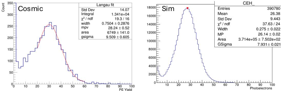
Fig: Typical PE distribution from UMass cosmic stand (left) and simulation (right) with the prototype detector module **Ring 5**.
