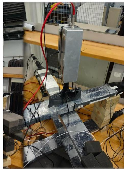
*Fig: (left) Pion detector prototype in MAMI e- beam , (right) prototype being tested in cosmic ray at jlab*
