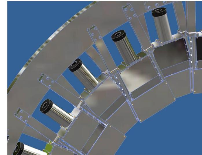
Fig: Shower-max detectors in its support ring
