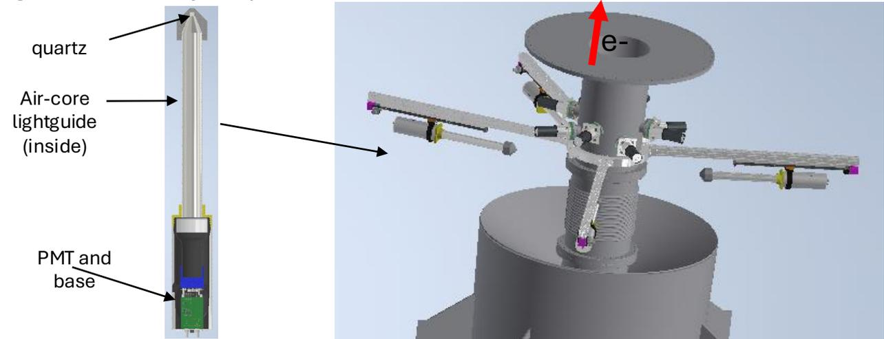
Fig: (left)CAD assembly of downstream scanner, (right) assembly around the beam line
