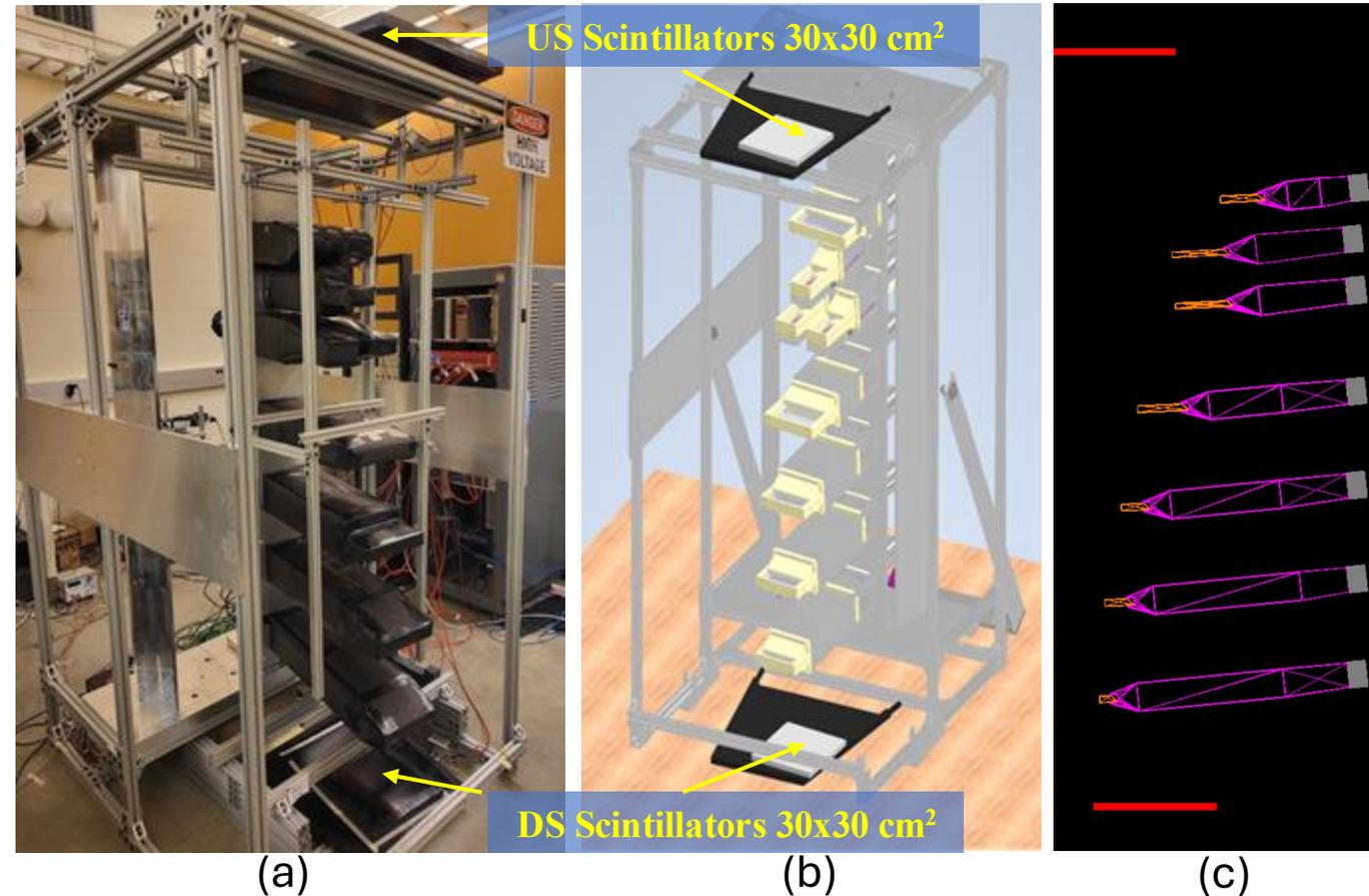
Fig: (a) UMass Cosmic stand taking data, (b) CAD model of the the same stand and (c) the visualization of the detectors from Monte Carlo simulation
