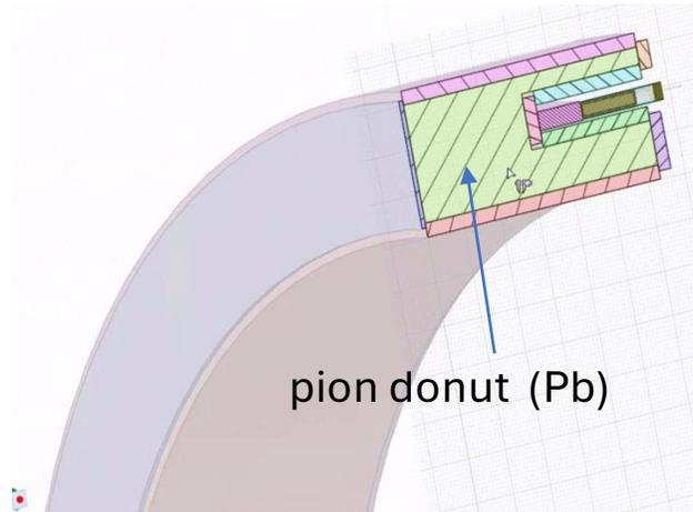
Fig: Cross section of the lead donut
