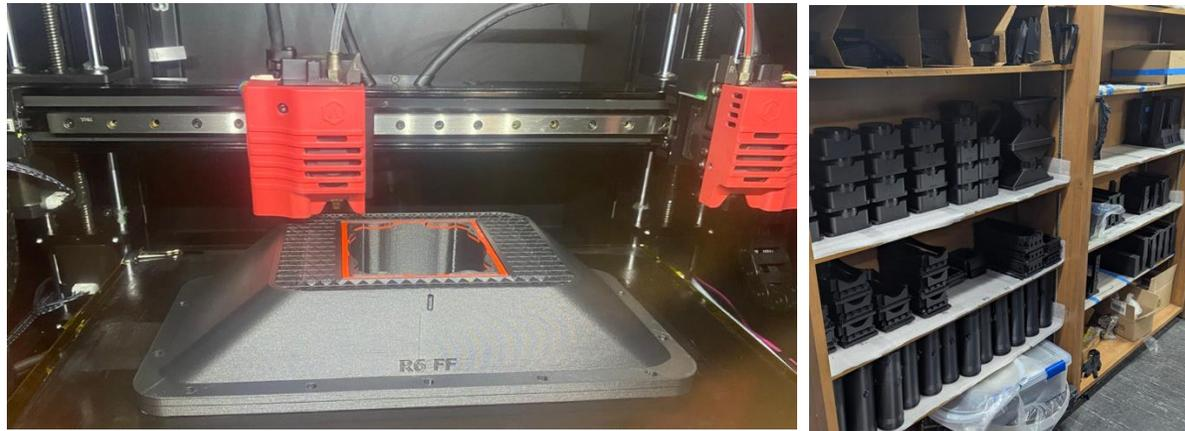
Fig: (left) Printing ring6 component, (right) printed parts on the shelf in cleanroom
