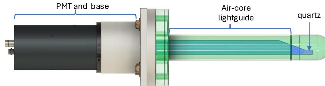
Fig: CAD model of SAM
