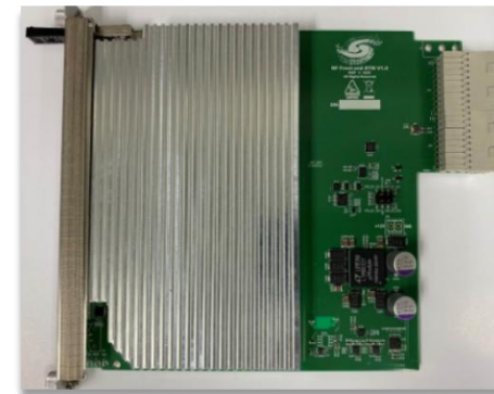
In-house made DWC RTM 2856MHz
