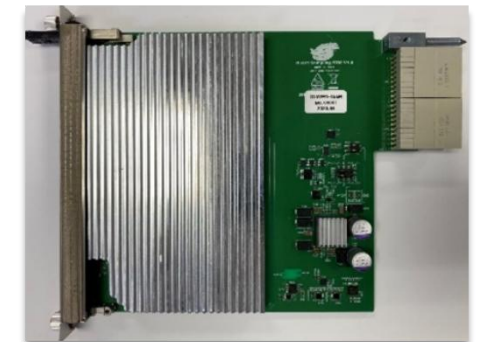
In-house made DS RTM 142.8/571.2MHz
