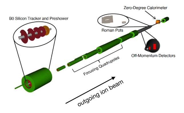
Charged hadrons: Forward spectrometer Neutral hadrons: Zero-Degree Calorimeter
