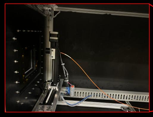
A translation stage in dark box allows a pulsed LED to scan pixels of detector
