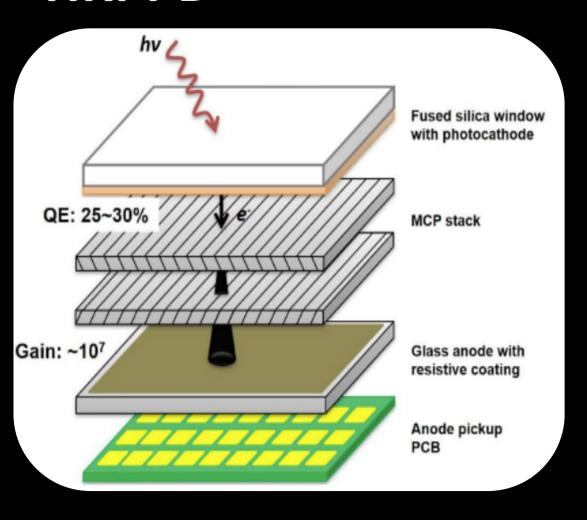
Incident photons dislodge an electron from cathode
