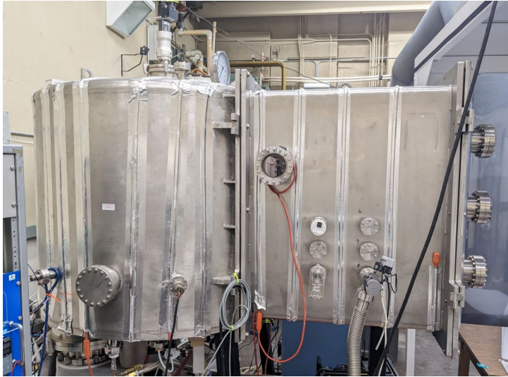
Evaporator Exterior with 10^{-6} torr vacuum capabilities
