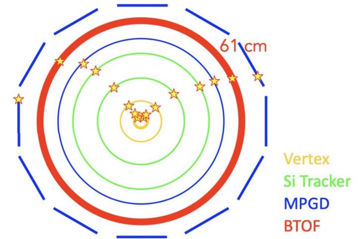
The tracking system from inside out: vertex, Si Tracker, MPGD, BTOF
