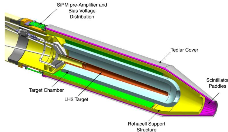
Fig. 1. The GlueX Start Counter mounted to the liquid H<sub>2</sub> target assembly. The beam direction is oriented from left to right down the central axis of the ST.
