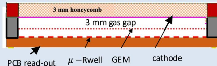
$\mu$ Rwell as spin off of the high-lumi project (various prototypes up to 40 x 46 cm<sup>2</sup> exist)
