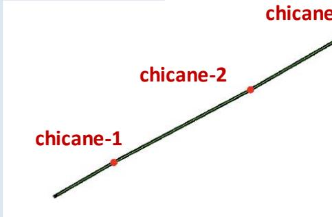
Beam pipe + 1 cm lead in the proper locations suppress synchrotron radiation to a negligible level
