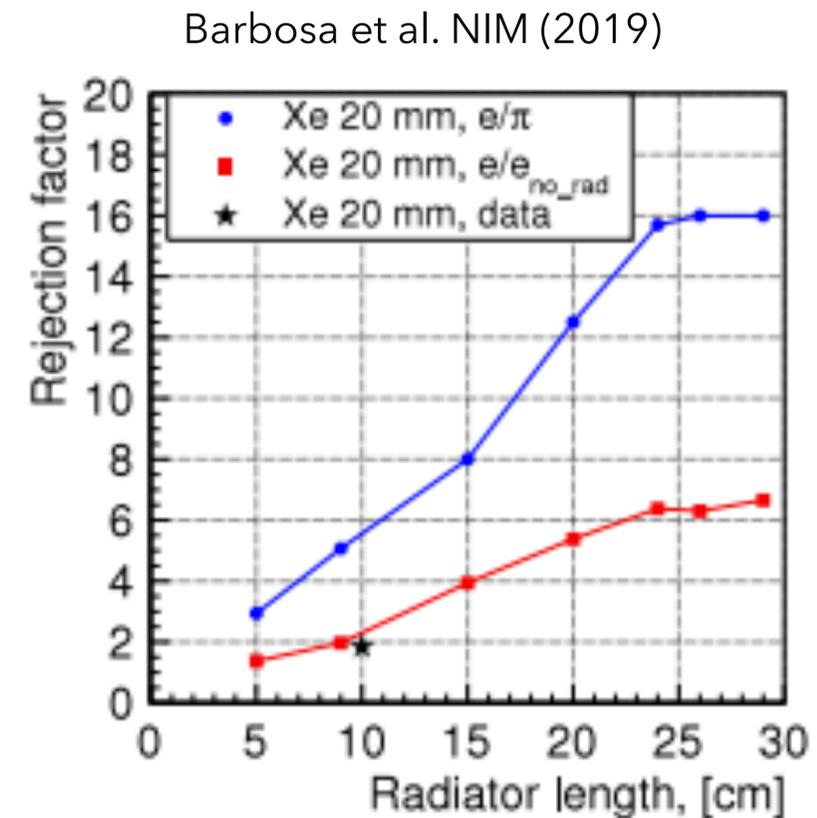
**Planned 15-cm forward TRD provides  $\sim 10\times \pi^\pm$  rejection**
