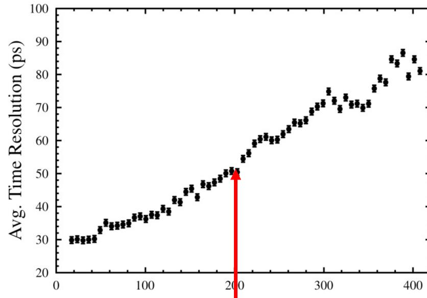
With a 200-cm-long detector and 3 MeV threshold ( $\sim 5\%$  neutron efficiency), projected time resolution is 100 ps.
