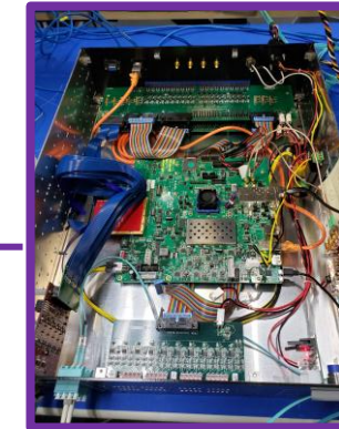
Global Timing Module (NSLS II/sPHENIX) Receiving from RHIC RF low jitter clock source
