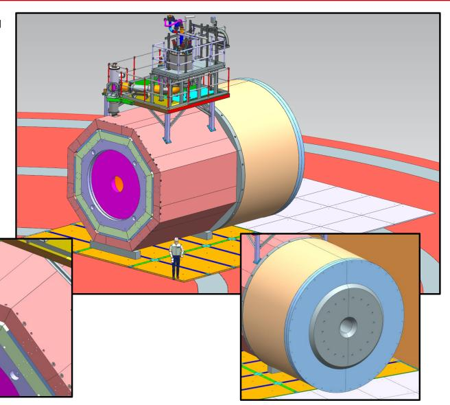
Downstream end of the magnet – endcap removed
