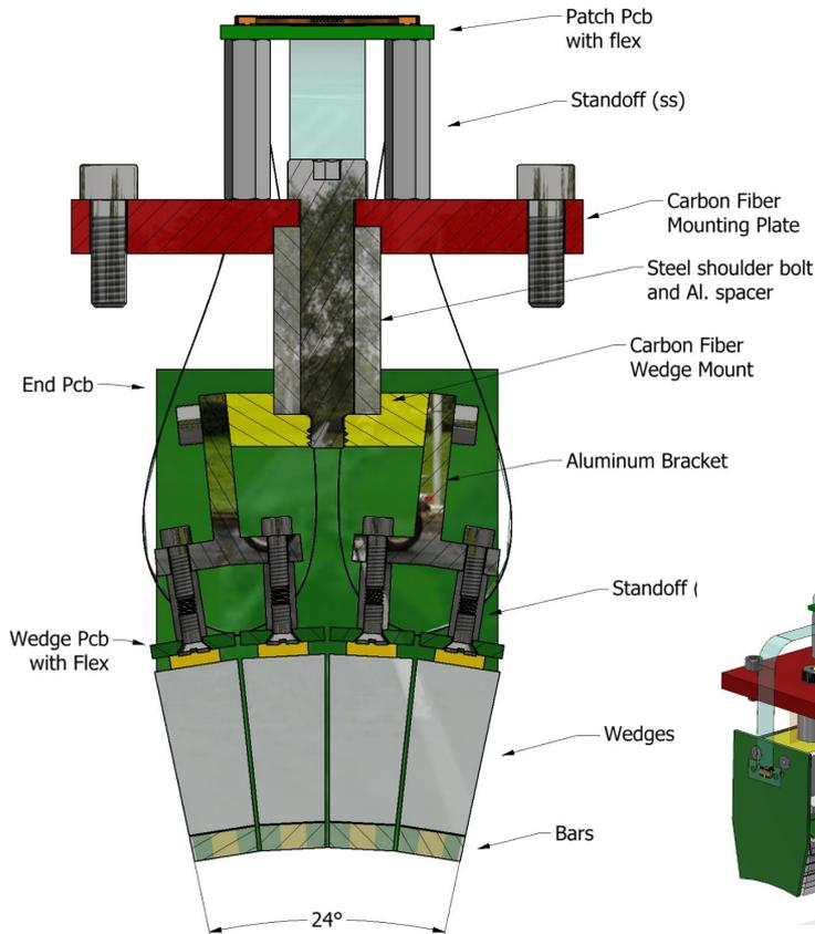
Inner bar thickness : 3 mm. Outer wedge thickness : 2 cm.
