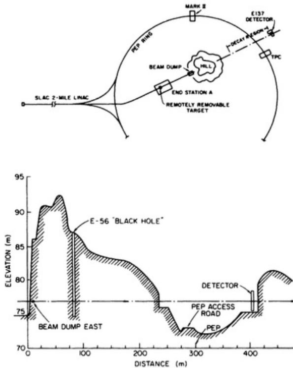
FIG. 2. Layout of SLAC experiment E137.
