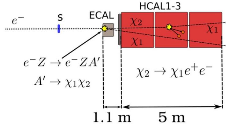
**Fig. 3** A schematic view of an event  $A' \rightarrow \chi_1 \chi_2 (\chi_2 \rightarrow \chi_1 e^+ e^-)$  from a  $A'$  produced after a 100 GeV  $e^-$  scatters off in the active dump,  $e^- Z \rightarrow e^- Z A'$ . The  $\chi_2$  particle decaying within HCAL2 corresponds to the S1 signature (see text for more details)
