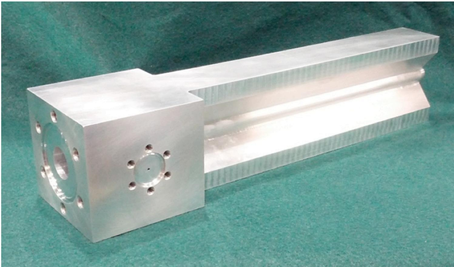
Relatively small amount of tritium ( $\sim 1\text{kC}$ ) in a cell machined from single block of Al.
