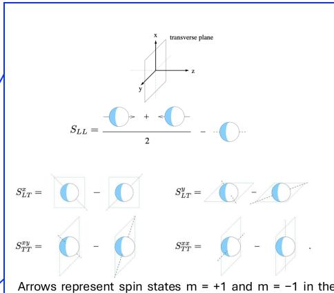
Arrows represent spin states m = +1 and m = -1 in the direction of the arrow itself, while dashed lines denote spin state m = 0 again in the direction of the line itself
