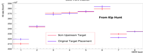
Impact on GEM background rate (GEP-3, Q^2 = 12.04 \text{ GeV}^2 ), Front Tracker SBS front tracker
