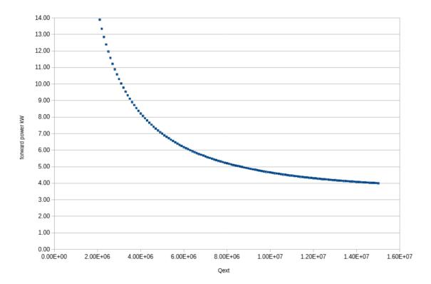
Adapted from spreadsheet provided by C. Giovati 6 kW from klystron 5.2 kW usable at cavity
