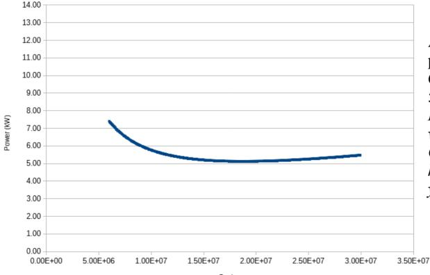
Adapted from spreadsheet provided by C. Giovati 6 kW from klystron 5.2 kW usable at cavity Design goal: 19 MV/m with 8 kW klystrons. Circulators needed to run klystrons at 8 kW are not yet available.
