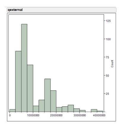
Coupling of power from the klystron to the cavity and beam is determined by Qexternal. Power  $\sim V^2/Qext + I^2*Qext + microphonics$ .
