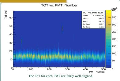
Coupled with the LE calibrations, we are able to use the ToT sum for observed clusters as an electron even selection (pion rejection).
