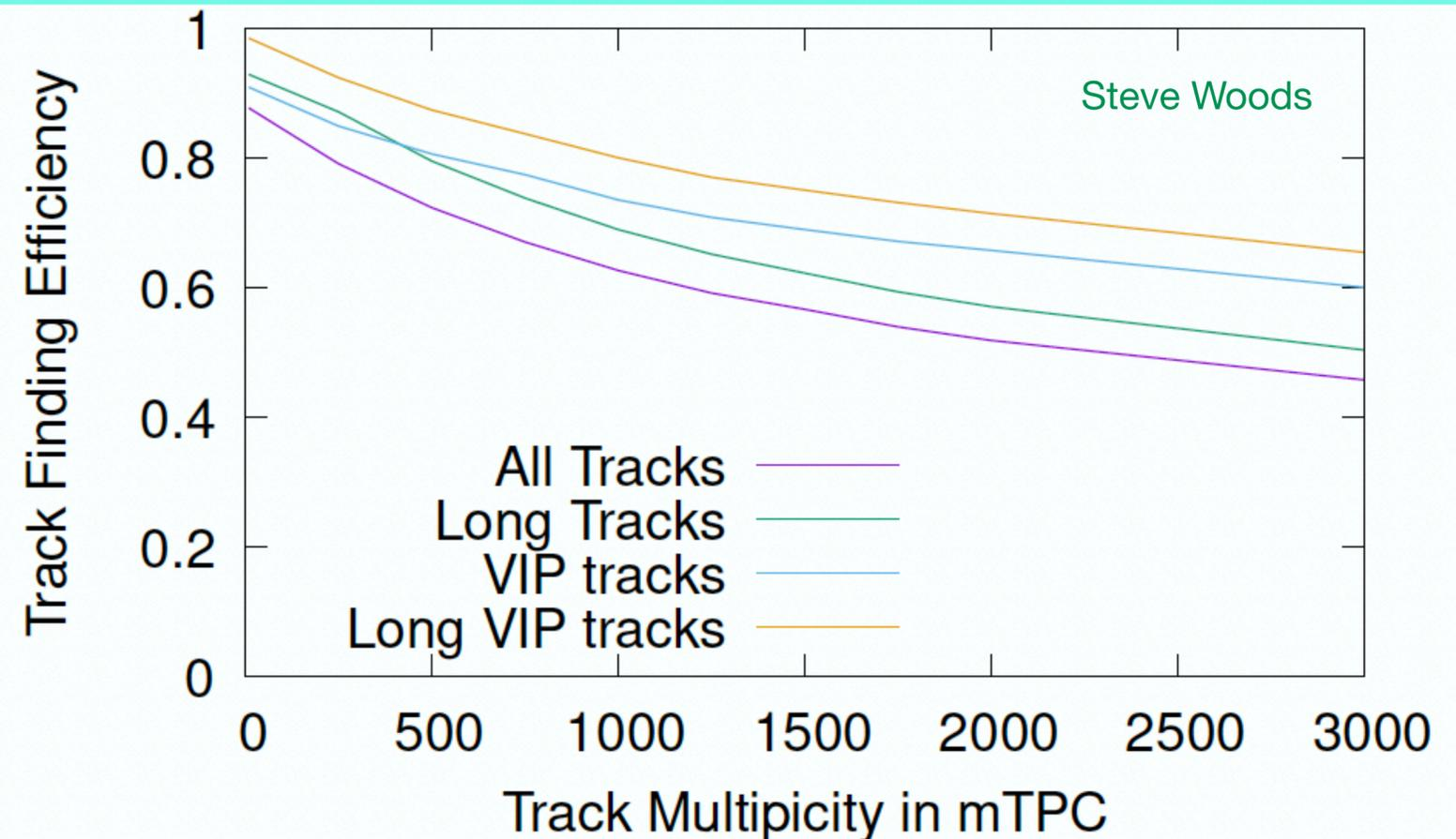
At multiplicity of 2000 tracks per event (~1GHz in entire mTPC volume) shows efficiency of 68% for clean tracks
