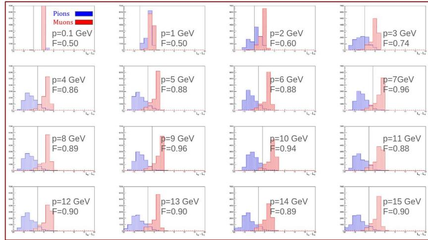
Ln(Likelihood) differences between muons and pions in single particle simulations in the EPIC detector using the barrel calorimeters
