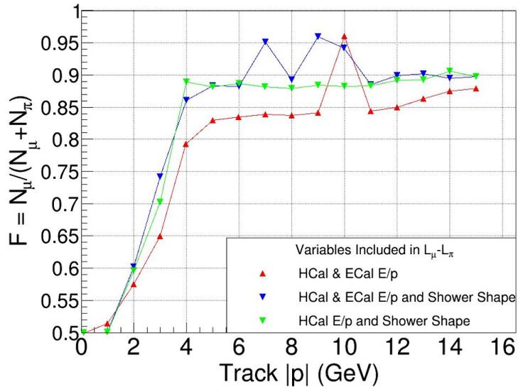
Purity of muons ( $N_{\mu} / (N_{\mu} + N_{\pi})$ ) based on example  $\ln(\text{likelihood})$  cuts.
