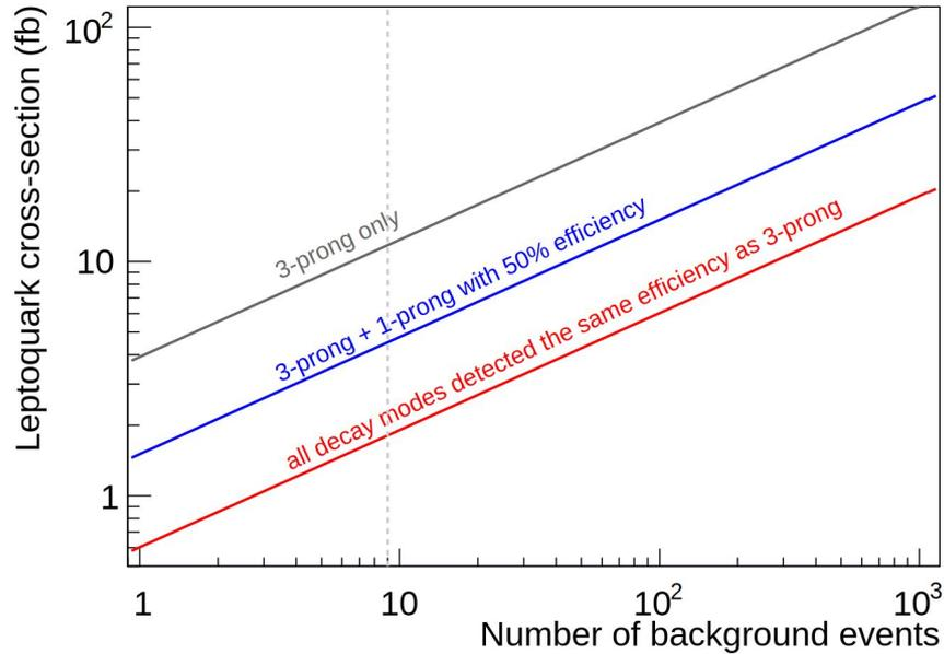
sensitivity for leptoquark cross section vs # remaining background
