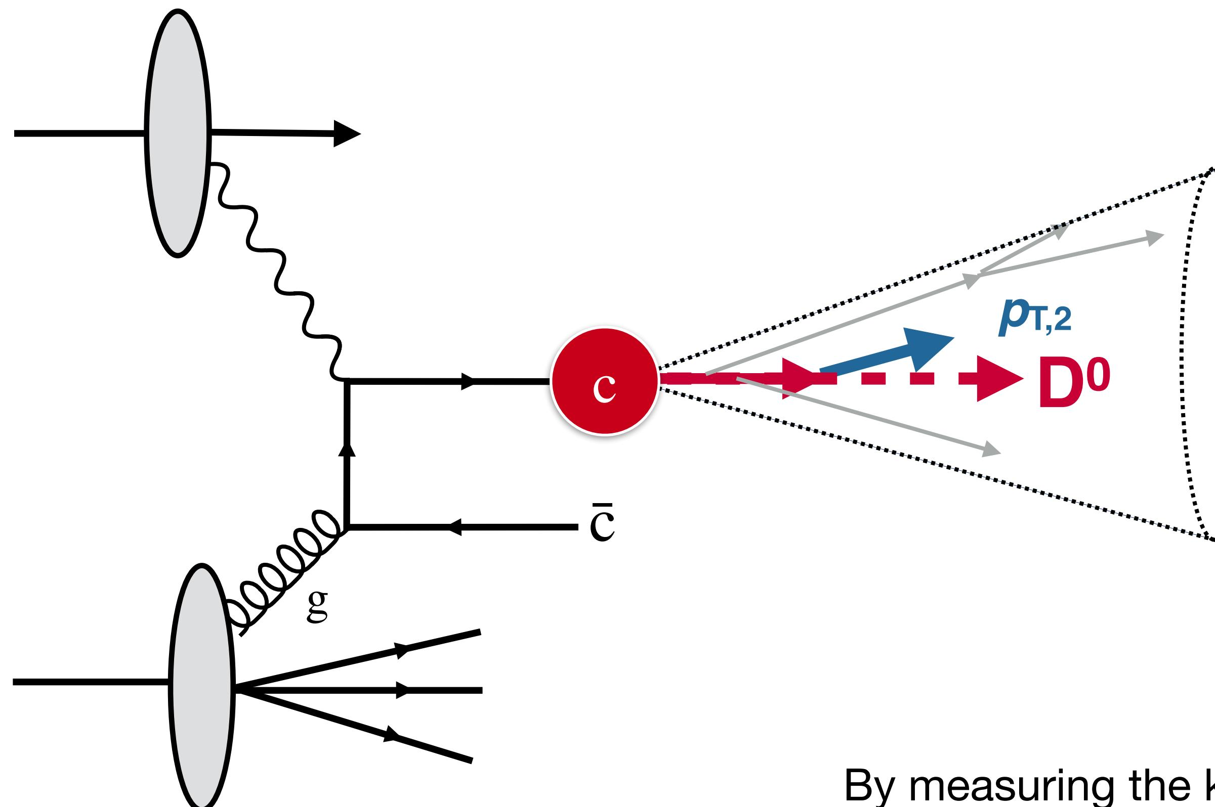
Jet-“reclustering” techniques to access with high accuracy the  $p_T$  of the associated charm jets
