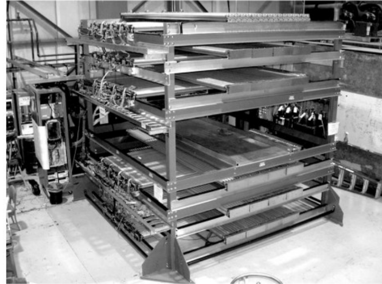
Example of straw tube chambers similar to Seaquest experiment
