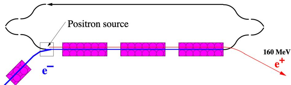
Figure 4: The layout for positron production at 160 MeV.
