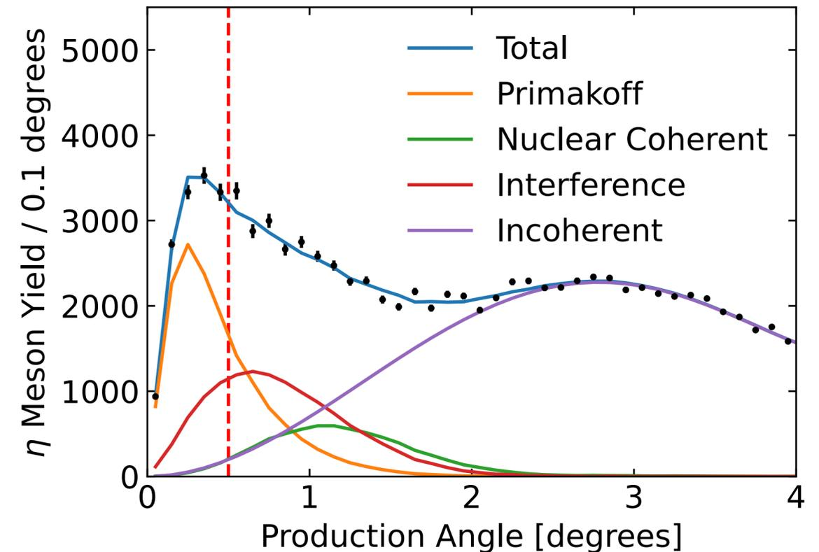
Angular distribution used to determine Primakoff contribution to  $\eta$  production
