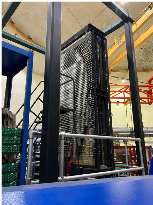
ECAL Rear view. Cooling system is installed.
