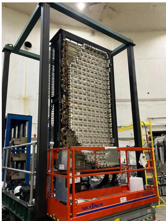
ECAL Front view. All Supermodules (1700 blocks) installed. Installing heaters
