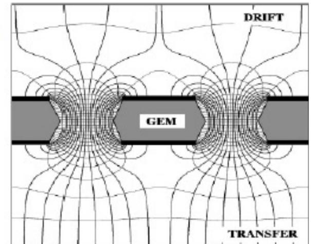
Figure 54. Electric field and equipotential lines in the gas electron multiplier.
