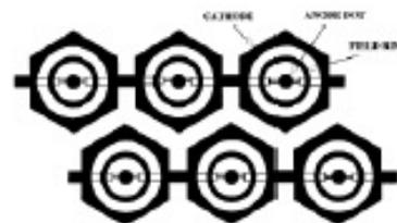
Figure 26. Schematic of the microdot chamber: A. pattern of metallic anode dots surrounded by field and cathode electrodes is implemented on an insulating substrate, using microelectronic technology. Anodes are interconnected for the readout.
