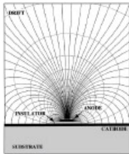
Figure 21. Elemental and electric field lines for the micro-gap chamber.
