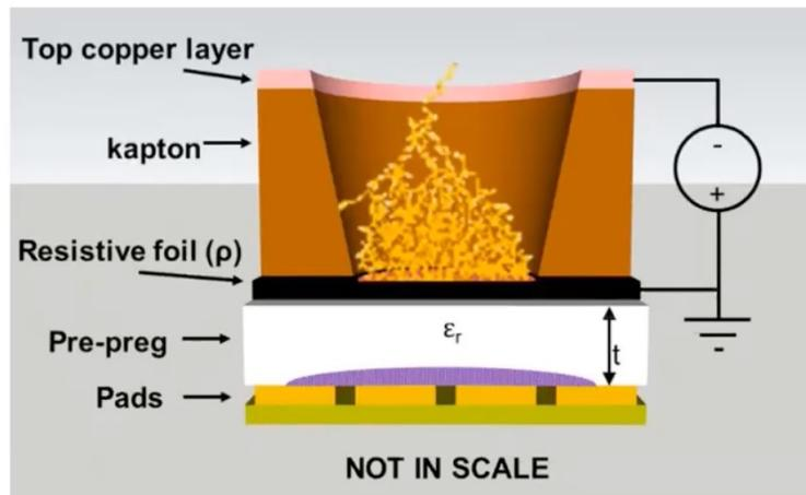
Applying a suitable voltage between the **top Cu-layer** and the **DLC** the WELL acts as a **multiplication channel for the ionization** produced in the conversion/drift gas gap.
