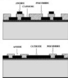
Figure 25. Two variants of micro-gap chambers, using thick polyimide ridges to prevent the onset of discharge.
