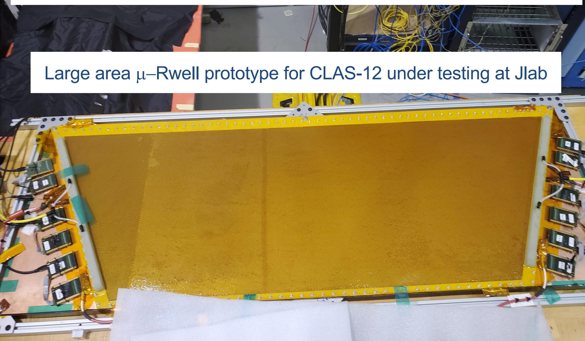
Large area  $\mu$ -Rwell prototype for CLAS-12 under testing at Jlab
