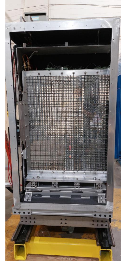
\text{PbWO}_4 crystals in copper frame
