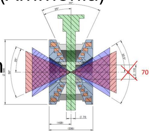
Cross-section through the magnet showing the beam and cold finger access diameters (in mm) and c
