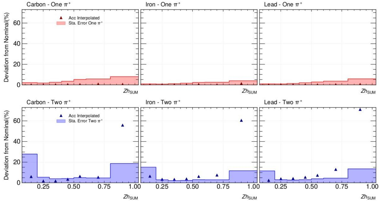
Figure 3.39: Deviation from the nominal  $\Delta P_t^2$  value due to do not interpolated the acceptance factors.
