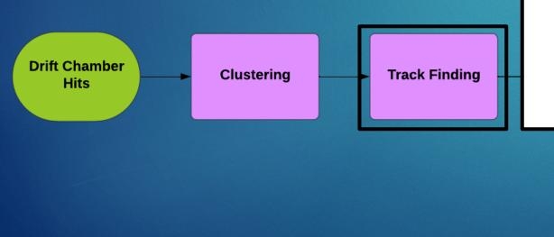
Track Finding as used in AI reconstruction. Track parameters  $(P_x, P_y, P_z)$  then used for physics.
