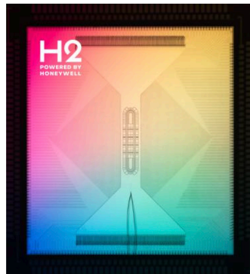
4 Logical Qubits 32-qubit H2-1 trapped ions (Quantinuum-Microsoft)
