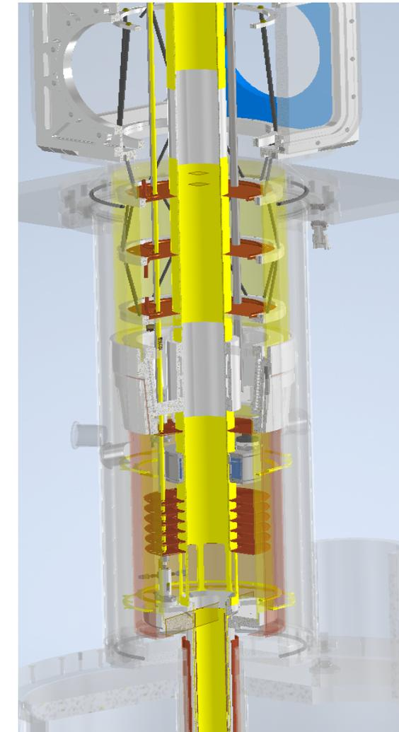
Cryomagnetics Cryo-Free 5 T Warm Bore Magnet
