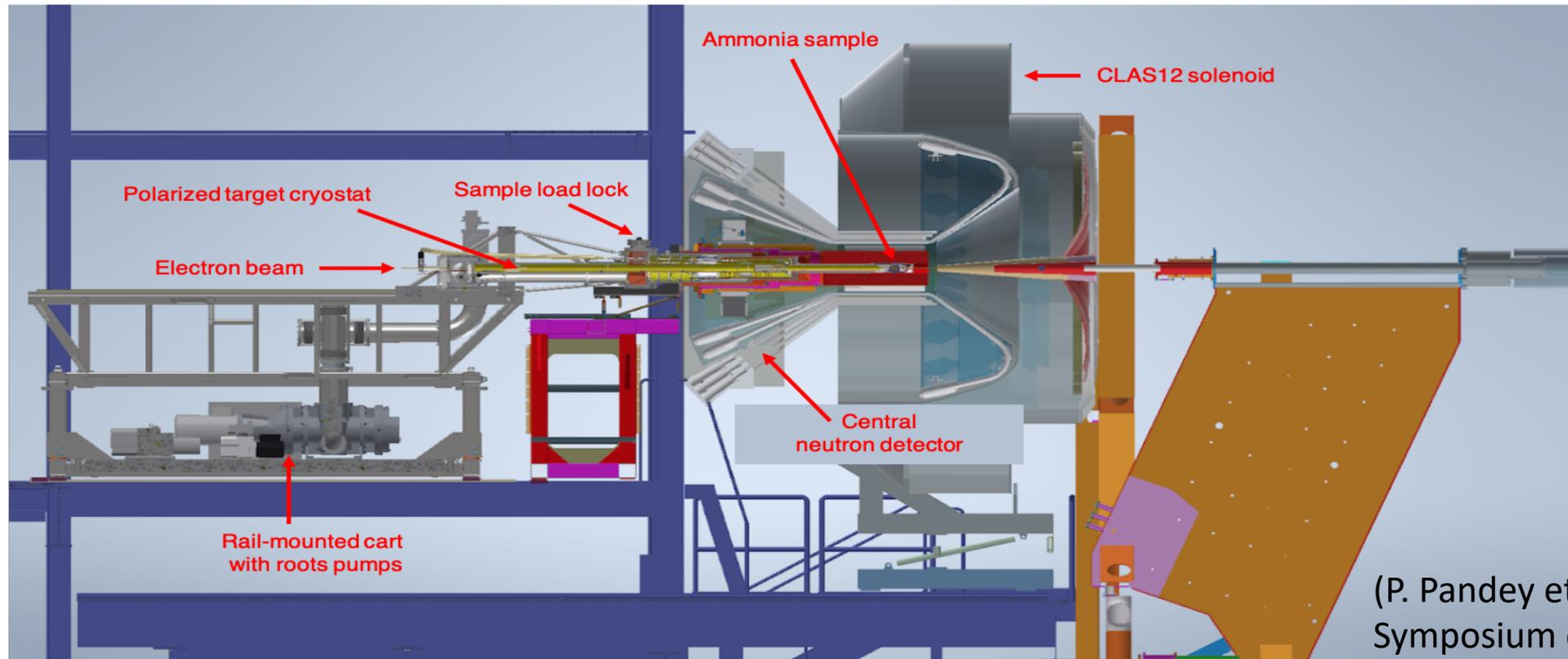
Side view of the polarized target installed in Hall B. A few elements of the CLAS12 spectrometer are shown.
