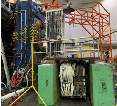
Inline SBS GEMs installed and tested during GEn
